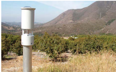
FIGURE 3: WILDFIRE DETECTOR. FIREALERT MK I DETECTS WILDFIRE OVER 1-MILE LINE-OF-SIGHT RADIUS.
